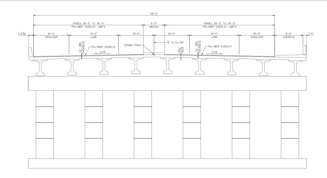
TYPICAL SECTION THRU S.T.H. 144 54W" PRESTRESSED CONCRETE GIRDERS (LOOKING NORTH)
