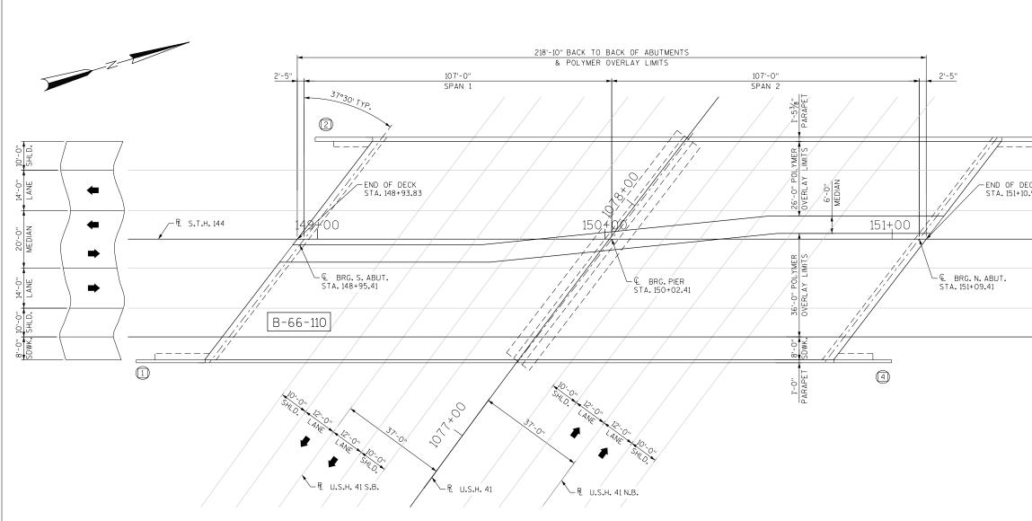
POLYMER OVERLAY FOR 2-SPAN 54W" PRESTRESSED GIRDERS
