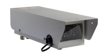
The light receptor measures the average luminance within an acceptance angle subtending  $20^{\circ}$ , (as recommended by CIE 088:2044 and RP-22-11), over a measurement range of 0 - 10,000 cd/m<sup>2</sup>, which can be scaled to suit customer requirements.
