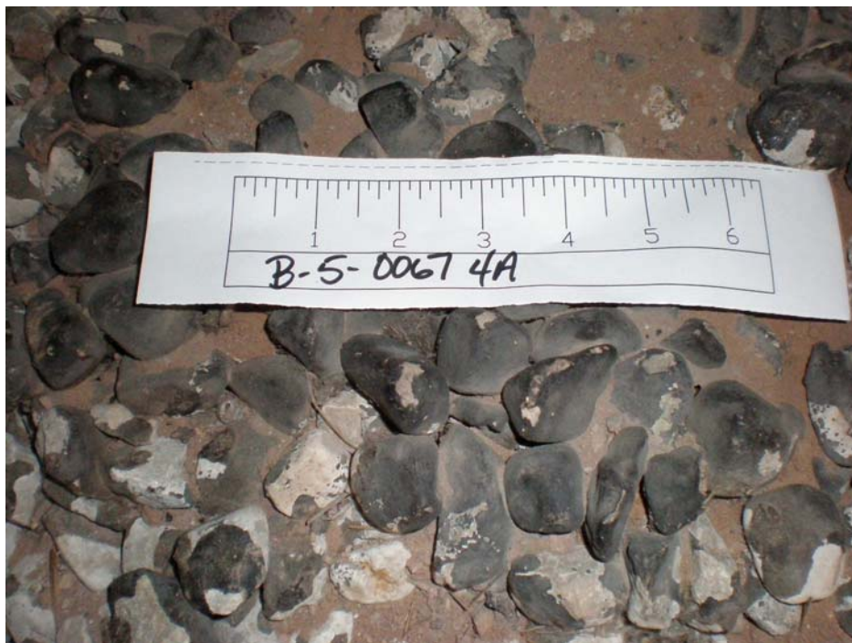
Tar covered rocks located beneath Structure B-05-0067.
