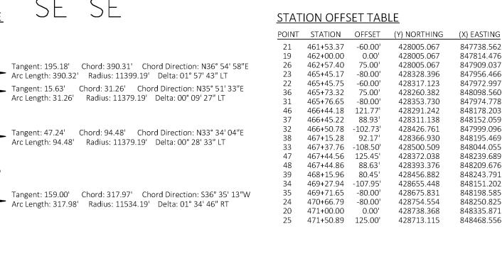
POSITIONS SHOWN ON THIS PLAT ARE WISCONSIN COUNTY COORDINATES, FOND DU LAC COUNTY, NAD83 (91) IN U.S. SURVEY FEET. VALUES SHOWN ARE GRID COORDINATES, GRID BEARINGS AND GRID DISTANCES. GRID
