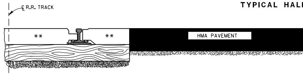
SECTION A-A HMA PAVEMENT APPROACH
