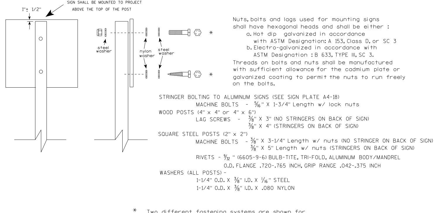
Two different fastening systems are shown for illustration purposes. On any individual sign, either one or the other system shall be used. Actual number of fasteners per sign varies with the sign area, but normally there are two. For a single post installation, all signs greater than 9 sq. ft. require the use of 3 fasteners.
