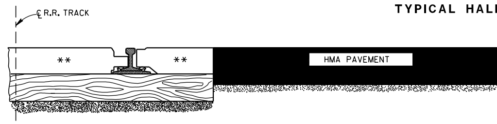
SECTION A-A HMA PAVEMENT APPROACH
