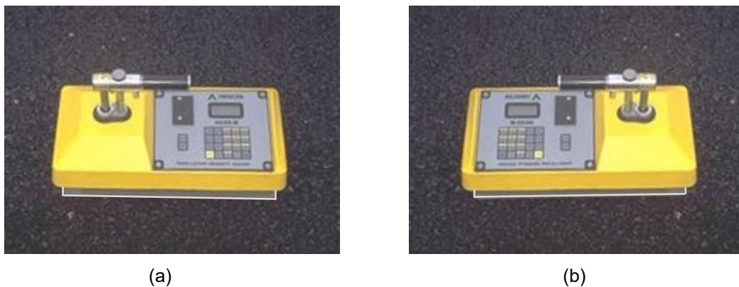
Figure 2: Nuclear gauge orientation for (a) 1 st one-minute reading and (b) 2 nd one-minute reading
