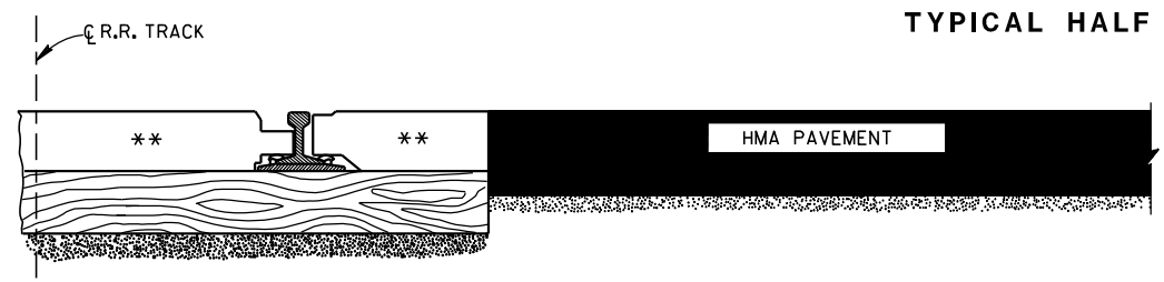
SECTION A-A HMA PAVEMENT APPROACH
