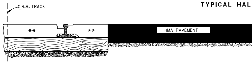
SECTION A-A HMA PAVEMENT APPROACH
