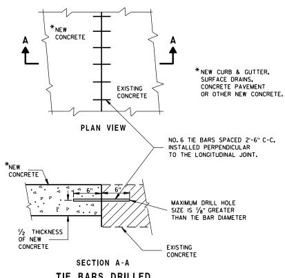
TIE BARS DRILLED INTO EXISTING PAVEMENT
