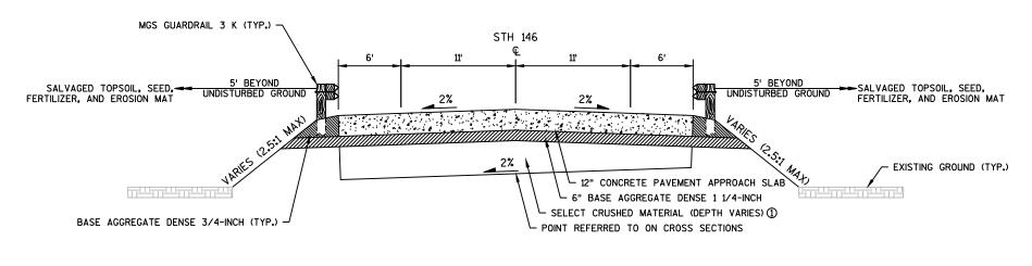
① SELECT CRUSHED MATERIAL FROM STA. 44+95.43 TO STA. 45+25.15 WILL SLOPE TO THE LEFT.
