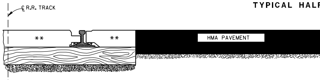
SECTION A-A HMA PAVEMENT APPROACH
