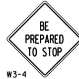
USE OF THE "BE PREPARED TO STOP" SIGN IS OPTIONAL. WHEN USED, THIS SIGN SHALL BE LOCATED BETWEEN THE W20-7a AND W20-4 SIGNS. A 500' TYPICAL SPACING SHALL BE PROVIDED BETWEEN THE SIGNS.
