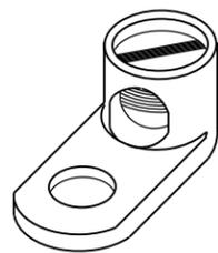
**TYPICAL MECHANICAL CONNECTOR LUG**
