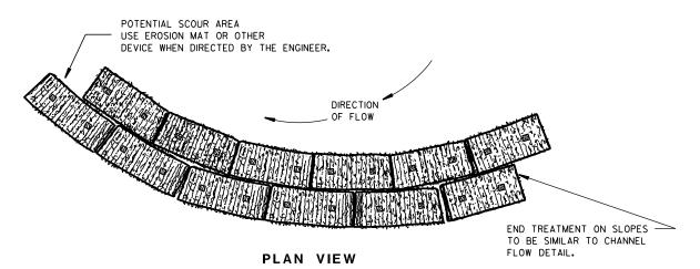
WHEN ALTERING THE DIRECTION OF FLOW
