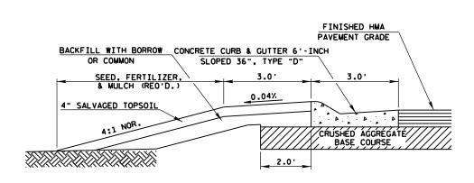
BERM DETAIL BEHIND 36" SLOPED CURB & GUTTER
