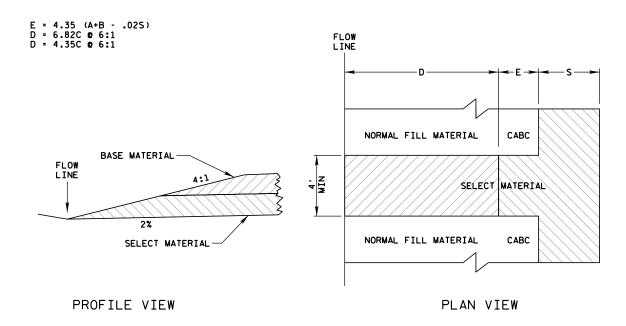
RELIEF TRENCH DETAIL CONSTRUCT RELIEF TRENCH AT SAG POINTS OR EVERY 250 FEET
