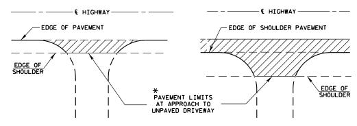
\* IF DRIVEWAY IS PAVED, APPROACH PAVEMENT TO BE EXTENDED TO MATCH DRIVEWAY PAVEMENT.
