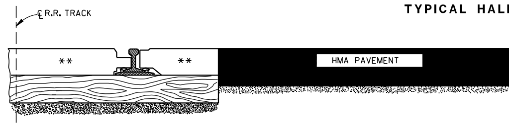
SECTION A-A HMA PAVEMENT APPROACH
