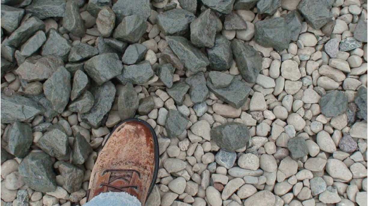
Figure 4.5. Railroad ballast / CA-15 composite base
