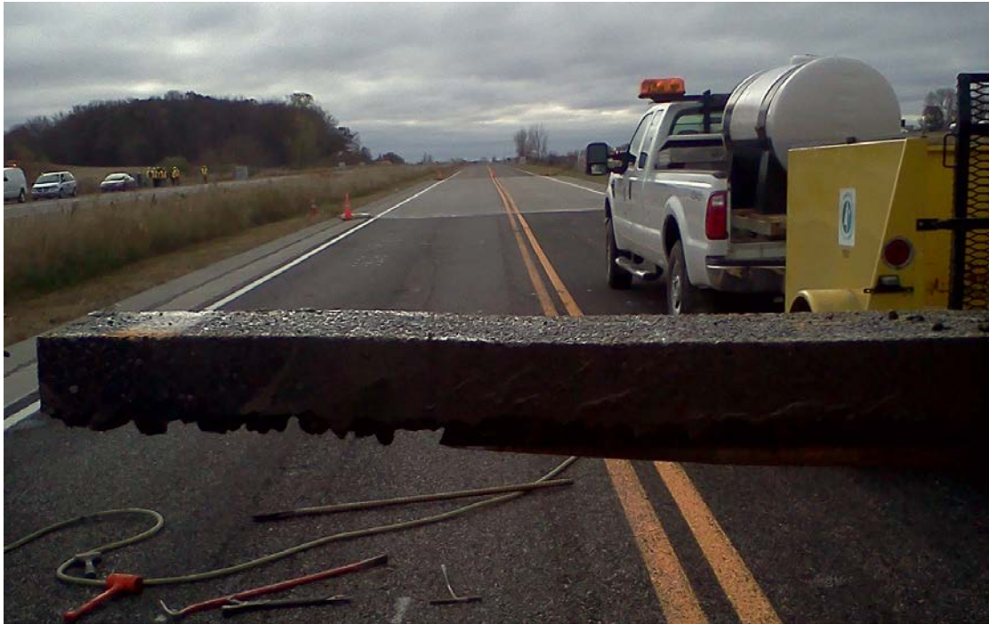
Figure 5.20. Forensic pavement section removed
