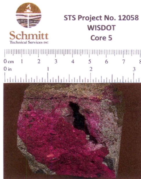
Figure 8. Core "5" showing a 35 mm (1.4 in.) deep by 5-to-15 mm (0.2-to-0.6 in.) wide void at a depth of 13 mm (0.5 in.) from the top of the core. Core top is toward top of photograph. This figure also illustrates the depth of carbonation from the wearing surface which is 25 mm (1.0 in.). Top scale is in millimeters and centimeters. Bottom scale is in inches.
