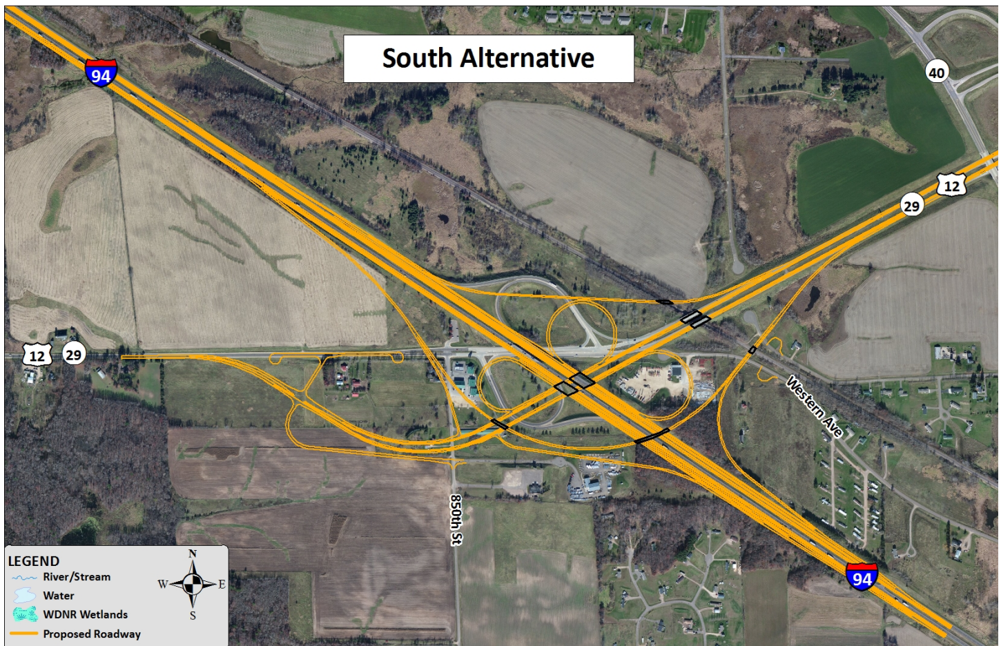
Figure 5: IH 94/US 12/STH 29 Interchange: South Reconstruction Alternative
