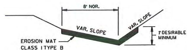
EROSION MAT DETAIL FOR DITCHES (SEE EROSION CONTROL PLAN FOR LOCATIONS) (REQ'D. IN ALL DITCHES)
