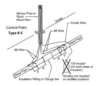
NOTE: ANODES ARE NOT REQUIRED FOR LOCATE POINTS ON THIS HIGH PRESSURE MAIN PER CORROSION GROUP
