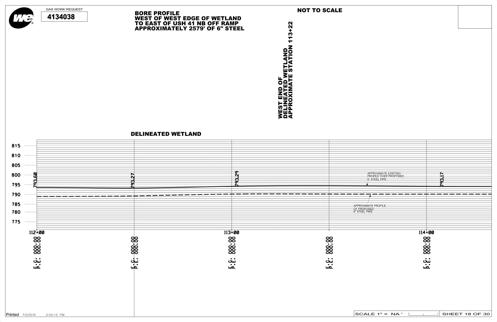
BORE PROFILE WEST OF WEST EDGE OF WETLAND TO EAST OF USH 41 NB OFF RAMP APPROXIMATELY 2579' OF 6" STEEL
