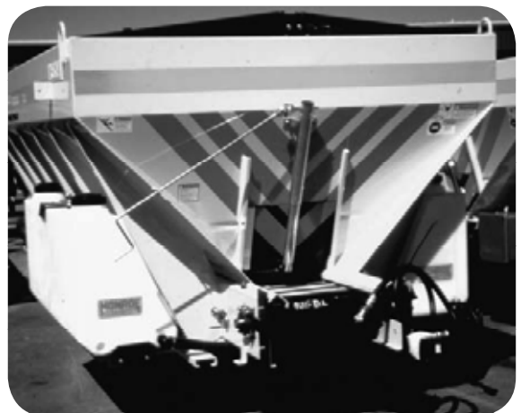
On-board prewetting using saddle tanks
